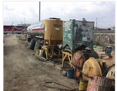
Inadequate secondary containment
